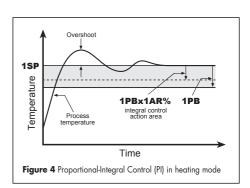
**4.3.3.** PROPORTIONAL-INTEGRAL-DERIVATIVE CONTROL. Response overshoot in a system controlled by a PI controller may be reduced by inserting a derivative action in the control. The derivative action is greater the faster the temperature variation within the time unit. A controller with a high derivative action (1DT high) is extremely sensitive to small temperature variations and can make the system instable. With 1DT=0 the derivative control is disabled.
